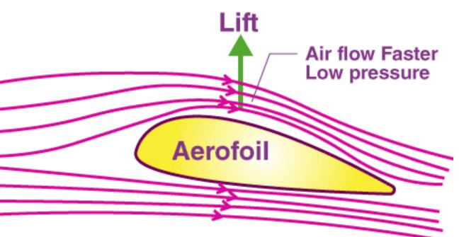
The asymmetric shape of an airplane's wing also generates the Magnus Effect, which can create lift.
